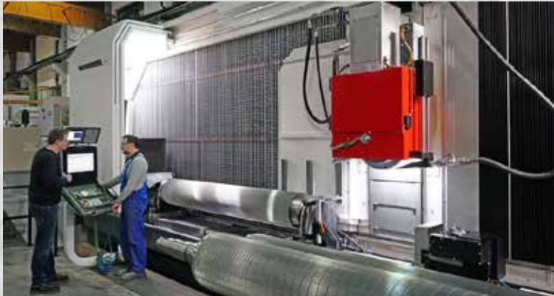
Corrugating grinding center, Ø 700 x 5000 mm
